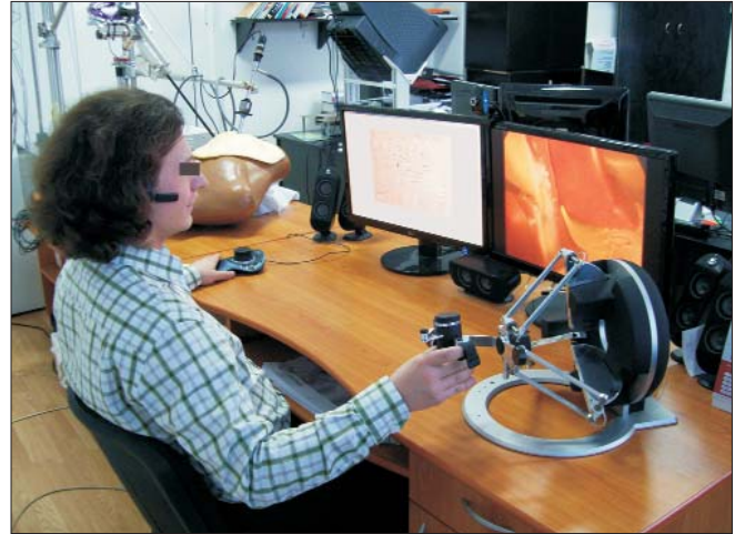
Figure 8. The robots PARMIS and PARASURG 5M controlled by voice, respectively by the haptic device
