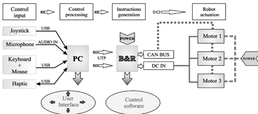
is presented in Fig. 5. The control input allows the user to give commands for the positioning of the laparoscope using different interfaces: joystick, microphone, keyboard & mouse and haptic device (Fig. 5).
