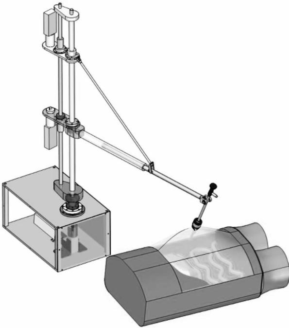
**Figure 1.** The virtual model of the PARAMIS parallel robot for MIS
