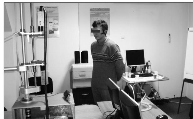
**Figure 7.** Voice controlled parallel surgical robot
