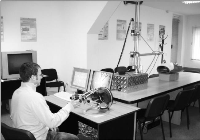
Figure 8. The robot control through the Joystick (haptic device)
